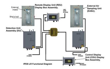
control functions, selects the state of the system, reports the system status, and provides audible and visual alarms upon detection.
