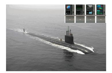
• A-RCI processes and displays the data from the LCCA. Combined with the legacy high-frequency sail array mounted in the front of the sail, LCCA provides the submarine crew with a near 360-degree high-frequency passive sonar capability. The LCCA is used to increase tactical control and situational awareness when operating in areas that are heavily populated with surface vessels.
