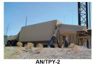
Mobile platform, variable orientation, phased array radars
