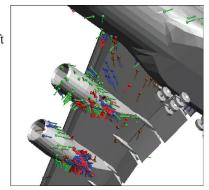
MANPADS engagement M&S facilities modeled specific MANPADS threats. A statistical comparison of the results and an analysis to validate MANPADS hit point prediction simulations was conducted. In FY11, the team will complete correlation of M&S hit point prediction test results with available live fire data, and develop a standardized methodology for hit point prediction simulations, improving MANPADS vulnerability analyses.
