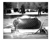
and a high-performance synthetic sealant that is one-fourth as dense as the natural gum rubber used in existing bladders. In FY10, METSS completed design verification testing including crash impact, gunfire, and panel testing. In FY11, the team will work with the U.S. Army Aviation Engineering Directorate on approved designs and procurement plans for two AH-64 Apache helicopter lightweight fuel bladders, including qualification testing to meet appropriate military specifications.
