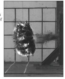
precursor and follow-through warhead effects on the target. Data from these tests will also give operational commanders better information on weapon effectiveness against targets in theater by including a wide variation of brick strengths in the target set.
