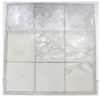
a prototype MH-47G helicopter down-look window with three times the viewing area of the current window that is 17 percent lighter and provides greater ballistic protection and multi-hit visibility.
