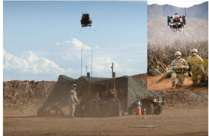
data terminal, an operator control unit, gimballed payloads (electro-optical or infrared), avionics pod, digital data link radios, electric fueler, and support equipment.
