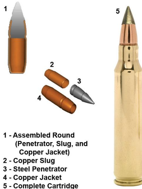
1 - Assembled Round (Penetrator, Slug, and Copper Jacket)
