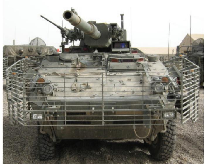
provided by add-on slat armor (high hard steel arranged in a spaced array).
