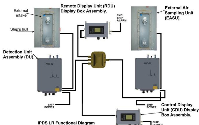
that provides the control functions, selects the state of the system, reports the system status, and provides audible and visual alarms upon detection.
