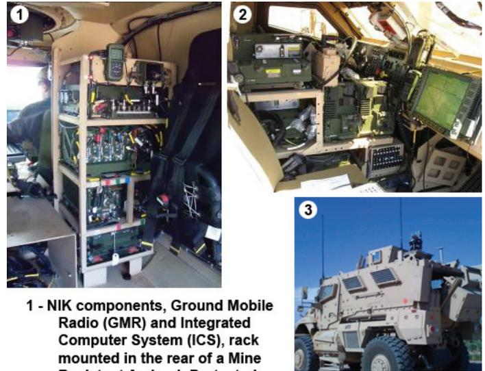
**1 - NIK components, Ground Mobile Radio (GMR) and Integrated Computer System (ICS), rack mounted in the rear of a Mine Resistant Ambush Protected (MRAP) vehicle**
