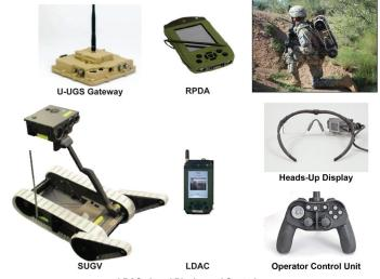
LDAC - Local Display and Control RPDA- Ruggedized Personal Digital Assistant SUGV - Small Unmanned Ground Vehicles U-UGS - Urban-Unattended Ground Sensors
