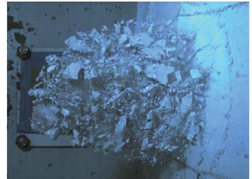
FATEPEN. FATEPEN is used to model fragments generated from fragmenting warheads striking concrete targets. This testing is focused on refined debris collection for concrete targets reinforced at various locations. FATEPEN is utilized by both the JTCG/ME and JASP for the analysis of fragmenting warheads.
