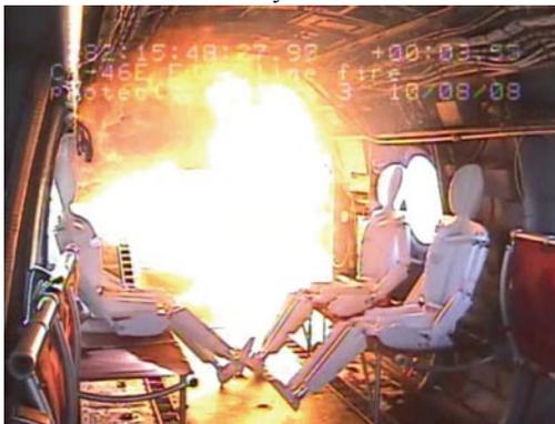
plastic sheets, and a low-cost, lightweight, commercial off-the-shelf (COTS) fire detection and extinguishing system known as the Firetrace Indirect Extinguishing system. Threats tested ranged from 7.62 mm armor piercing incendiary to 23 mm high explosive incendiary. The final report should be available through the Defense Technical Information Center by the end of 2009.
