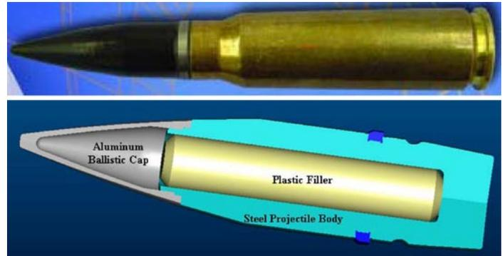
with very high pressure. The rapid expansion of the plastic filler ruptures the steel case, achieving fragmentation with lateral velocities of about 300 meters per second.
