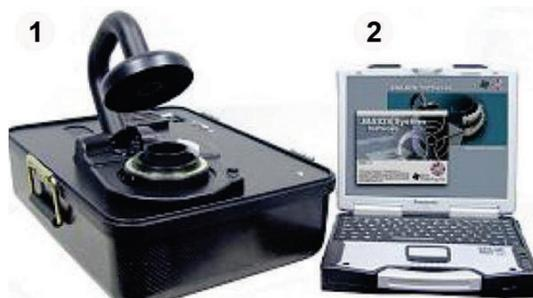
**1 - Polymerase Chain Reaction (PCR) Thermal Cycler**
