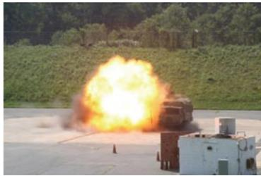
Instrumentation characterized the applied air-blast load to the target. Engineers then analyzed the data to develop lethal miss distance contours (the distance from a detonation that a person or equipment must be to survive) with respect to mobility, firepower, and catastrophic target kills.
