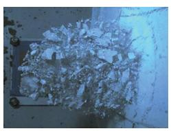
FATEPEN. FATEPEN is used to model fragments generated from fragmenting warheads striking concrete targets. This testing is focused on refined debris collection for concrete targets reinforced at various locations. FATEPEN is utilized by both the JTCG/ME and JASP for the analysis of fragmenting warheads.
