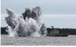
decommissioned Finnish fast attack craft. The Finnish Navy is providing the boats, and has conducted testing on their test range; the German and U.S. Navies are providing instrumentation, test planning, and analysis. The objective is to understand the behavior of aluminum structures subjected to various weapon effects; the ongoing validation of analytical tools for these applications is a primary objective.
