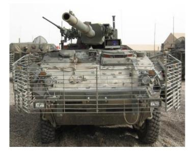
• The MGS provides the three-man crew with levels of protection against small-arms, fragmenting artillery, mines, and rocket-propelled grenades (RPGs). RPG protection is provided by add-on slat armor (high hard steel arranged in a spaced array).
