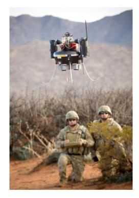
• The Class I Block 0 UAS takes off and lands vertically and once airborne uses both autonomous and manual flight mode navigation.
