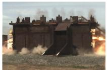
sizes were used. The Air Force Research Laboratory performed evaluations at the Reusable Target at Eglin Air Force Base. The Army Research Laboratory performed evaluations at the two-room blast structure at Aberdeen Proving Ground. The data obtained will be used to improve current methods for predicting weapon effects during Military Operations in Urban Terrain.
