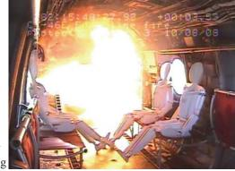
plastic sheets, and a low-cost, lightweight, commercial off-the-shelf (COTS) fire detection and extinguishing system known as the Firetrace Indirect Extinguishing system. Threats tested ranged from 7.62 mm armor piercing incendiary to 23 mm high explosive incendiary. The final report should be available through the Defense Technical Information Center by the end of 2009.
