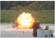
Instrumentation characterized the applied air-blast load to the target. Engineers then analyzed the data to develop lethal miss distance contours (the distance from a detonation that a person or equipment must be to survive) with respect to mobility, firepower, and catastrophic target kills.
