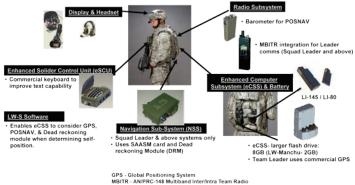
MBITR - AN/PRC-148 Multiband Inter/Intra Team Radio POSNAV - Position Navigation SAASM - Selective Availability / Anti-Spoofing Module
