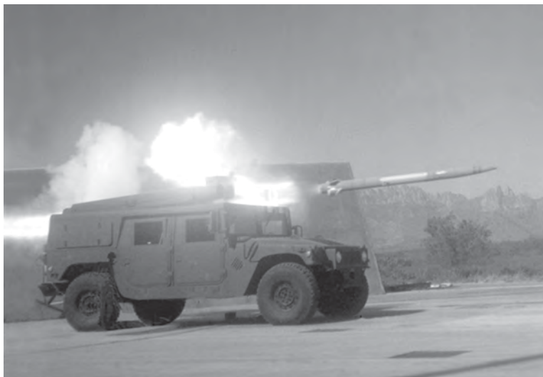
LOSAT is an antitank weapon system that fires a 177-pound penetrator rod munition.
