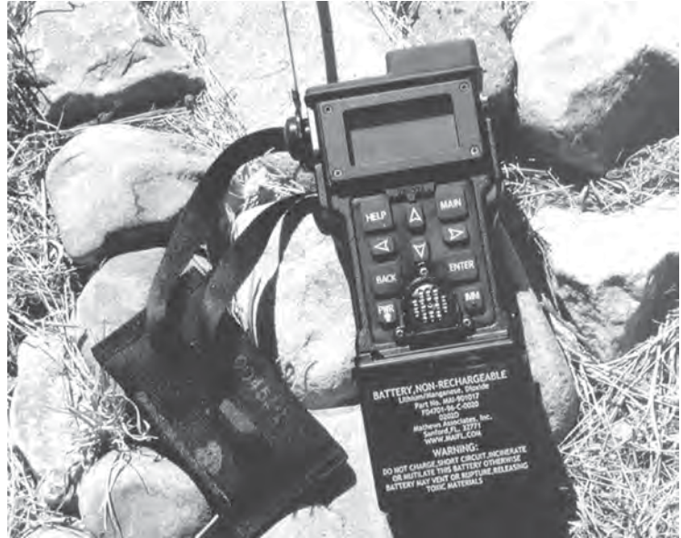
The hand-held radio uses line-of-sight UHF/VHF voice, rescue beacon, GPS, and over-the-horizon data modes for worldwide coverage.
