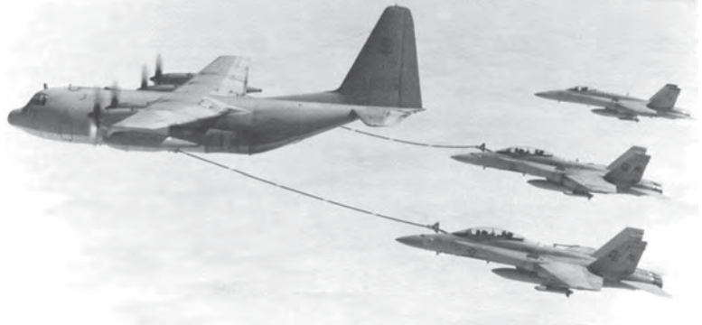
The KC-130J, a variant of the C-130J, is a medium-sized, four-engine turboprop aircraft modified to perform a primary mission of aerial refueling of fixed- and rotary-wing aircraft for the United States Marine Corps.
