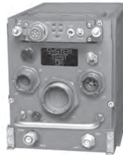
The IFF system is a cooperative question (interrogation) and answer (provided by a transponder) identification system.
