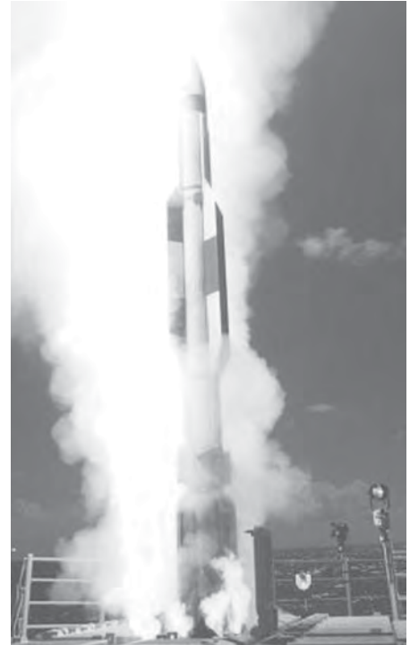
Given a command, the Aegis ship launches the three-stage SM-3 hit-to-kill missile and kinetic warhead.
