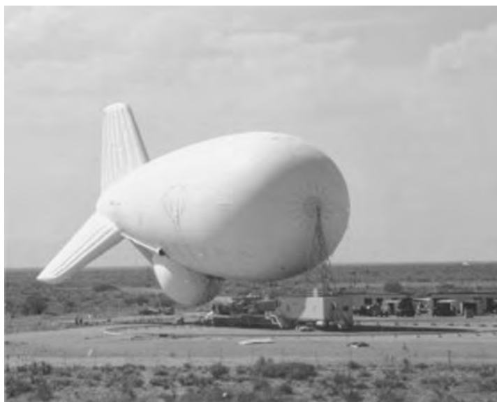
The Joint Land Attack Cruise Missile Defense Elevated Netted Sensor System is an airborne radar platform designed to provide surveillance and fire control quality radar data on Land Attack Cruise Missiles and other airbreathing targets.
