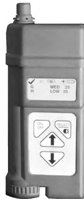
The Joint Chemical Agent Detector is a hand-held device that is intended to automatically detect, identify, quantify, and warn users of the presence of nerve, blister, and blood chemical agents.
