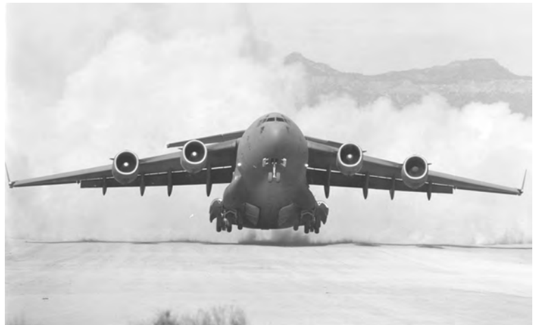
The C-17 carries outsize cargo and equipment over intercontinental ranges and is capable of delivery to austere airfields.
