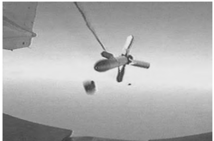
The Integrated Defensive Electronic Countermeasures is intended to provide increased self-protection and survivability for tactical aircraft against radio frequency and infrared surface-to-air and air-to-air threats. Current efforts are focused on radio frequency threats.
