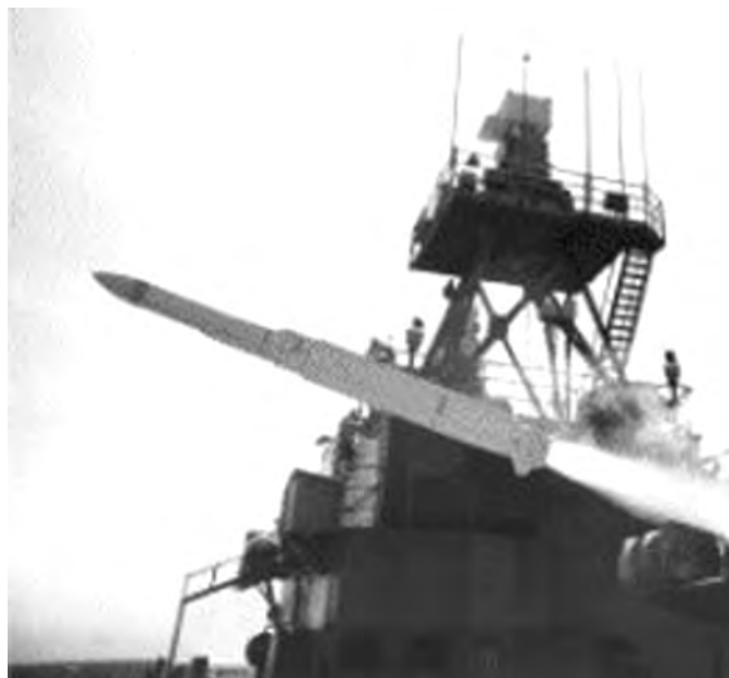
The Evolved Sea Sparrow Missile is a short-range missile intended to provide self-protection for surface ships.
