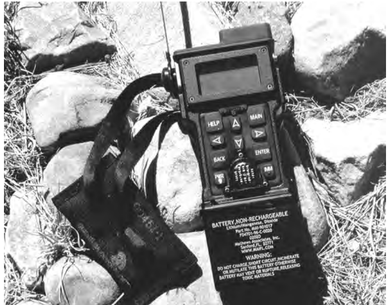
The Combat Survivor Evader Locator is a survival radio/personnel locator system designed to enable command elements and search and rescue forces to locate and maintain contact two-way communication with CSEL-equipped survivor/evaders.
