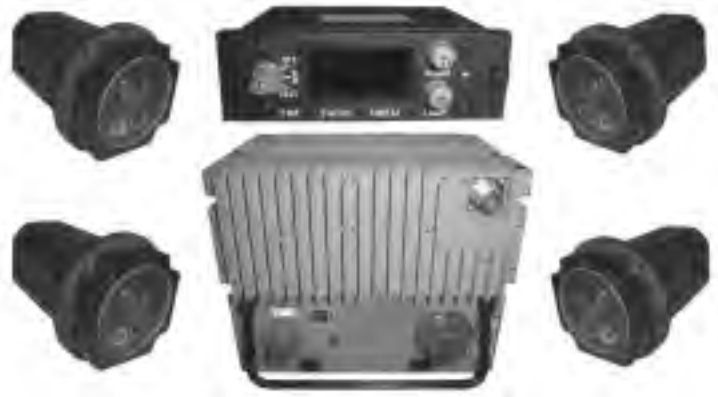
The original AN/AAR-47, fielded in the late 1980s, provides passive warning against infrared guided missiles directed at its host aircraft. The AAR-47(V)2 upgrade is intended to provide improved sensors that eliminate sensor blackening, increase temperature tolerance, and improve false alarm control.
