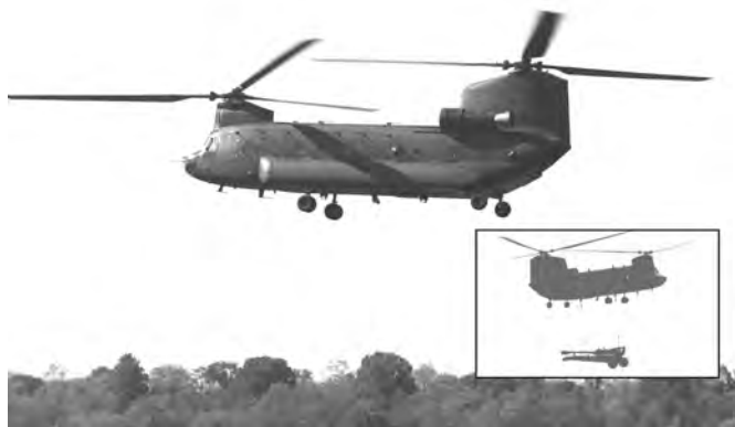
The CH-47 Improved Cargo Helicopter Upgrade performing external lift demonstration with an M-198 Howitzer.
