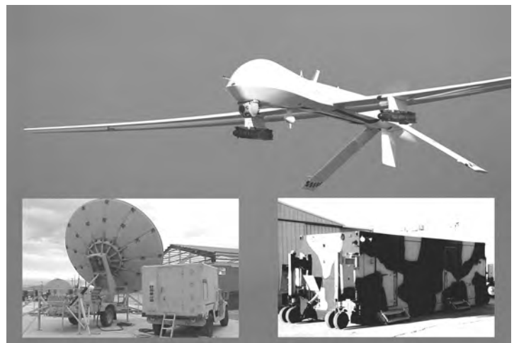
MQ-1 Predator: Originally designated RQ-1, multi-role systems capable of reconnaissance, surveillance, and limited strike are designated MQ-1.
