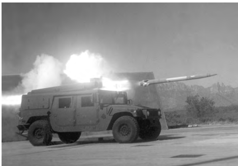
The Line-of-Sight Anti-Tank Missile is an anti-tank weapon system intended to provide lethal fire to defeat any known or projected armor system at ranges greater than 4,000 meters.
