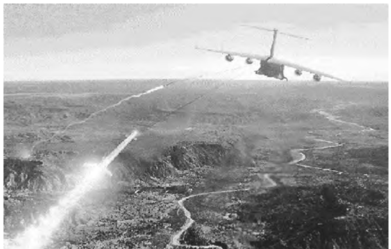
The Large Aircraft Infrared Countermeasures is designed to autonomously detect and declare Infrared threat missiles then track and jam the missiles.
