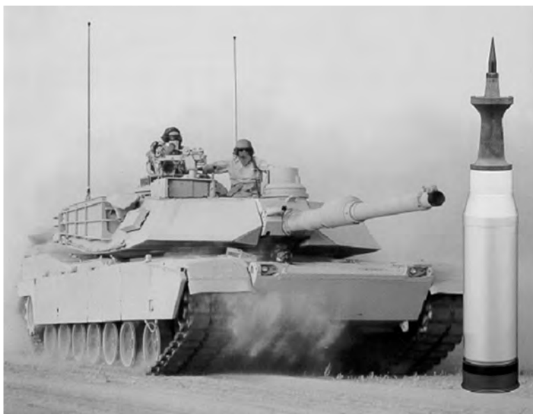
The M829E3 Armor-Piercing Fin-Stabilized Discarding Sabot-Tracer cartridge is a 120mm round designed to be fired from the Abrams tank.
