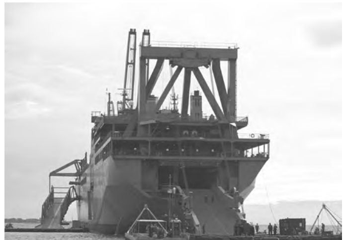
Strategic Sealift Ship preparing to embark tracked and wheeled vehicles through its extended stern cargo ramp.
