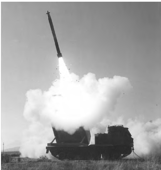
Guided Multiple Launch Rocket System is a guided rocket fired from the M270A1 or High Mobility Artillery Rocket System launchers. A unit equipped with GMLRS will shoot farther (60 km versus 30 km), achieve desired effects with fewer rockets (due to the improved accuracy), and have fewer duds than the currently fielded MLRS rocket.
