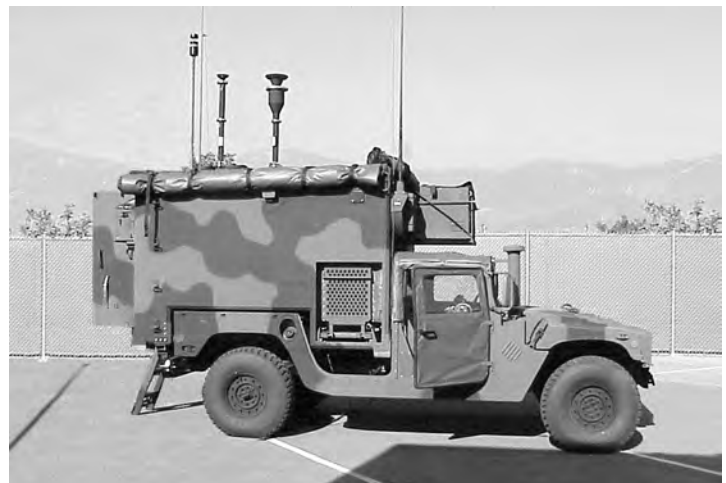
The Army's Joint Biological Point Detection System platform is the S788 lightweight, multi-purpose shelter mounted on a High Mobility Multipurpose Wheeled Vehicle - Heavy Variant.
