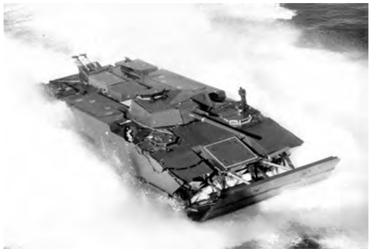
The Marine Corps' Advanced Amphibious Assault Vehicle underway at approximately 25 knots.
