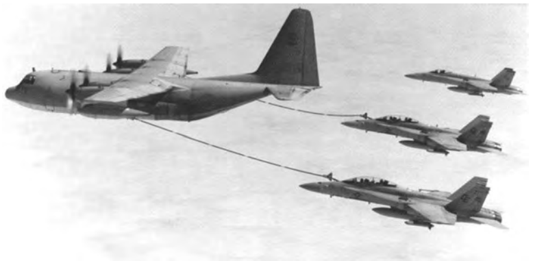
The KC-130J Marine Corps mission aerial refueling of fixed and rotary wing aircraft.
