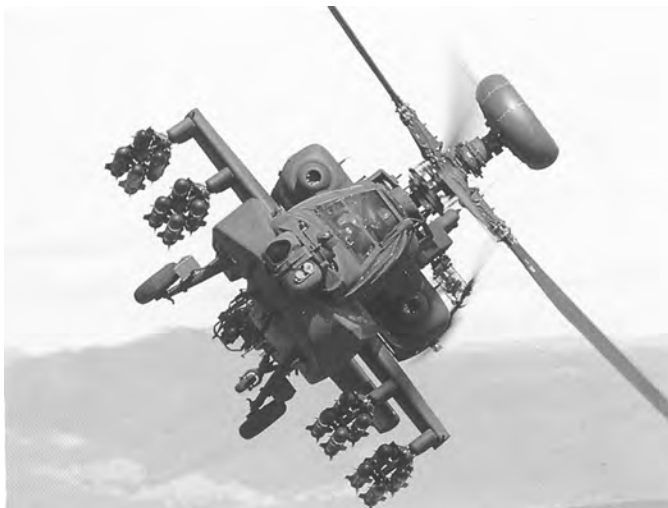
The Longbow Apache is a remanufactured and upgraded version of the AH-64A Apache Attack Helicopter.
