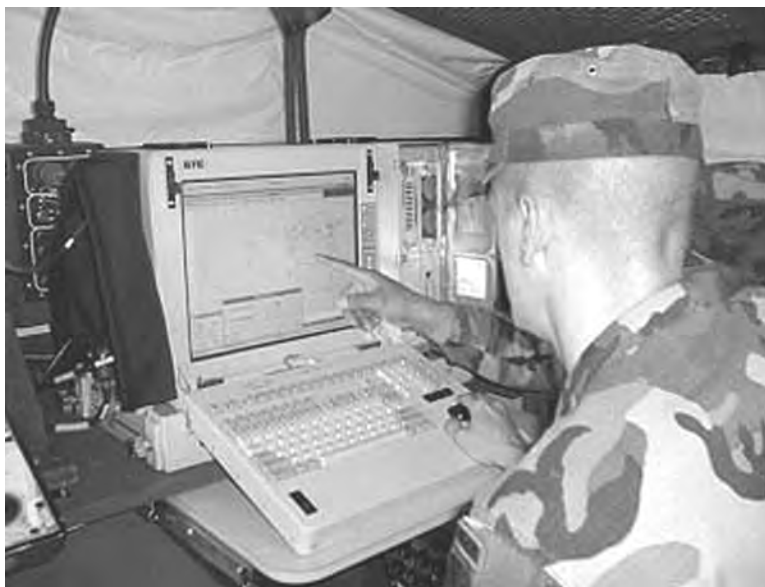
The Advanced Field Artillery Tactical Data System is a network of computer workstations that process and exchange information from the forward observer to the fire support element for all fire support assets (field artillery, mortars, naval gunfire, attack helicopters, and close air support).
