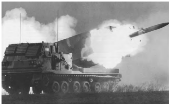
The launcher is the standard U.S. Army platform for firing surface-to-surface artillery rockets and missiles. The program includes two major upgrades to the current M270 launcher.
