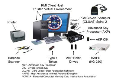
Key Processor for autonomous cryptographic key generation and a Type 1 user token for role-based user authentication. The commercial off-the-shelf components include a client host computer with monitor and peripherals, High Assurance Internet Protocol Encryptor (KG-250), printer, and barcode scanner.
